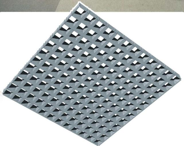
The U-profiles, orthogonally fitted, form modular panels complete with L perimetral profile for the support and the integration in the modular structure constituted by T profiles of 15 mm base. This system allows the use of different typology of panels but with the same module. Medi U-RASTER® can be supplied in a large range of standard cells end, on request, produced in various cell dimensions.
