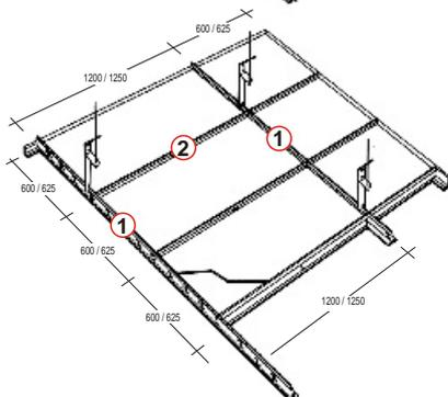
The 8T35 heavy exposed system, is constituted by heavy main runner and cross tees of mm. 1200 and mm. 600 hook system, with a dimension of all the system of mm. 35x38.
